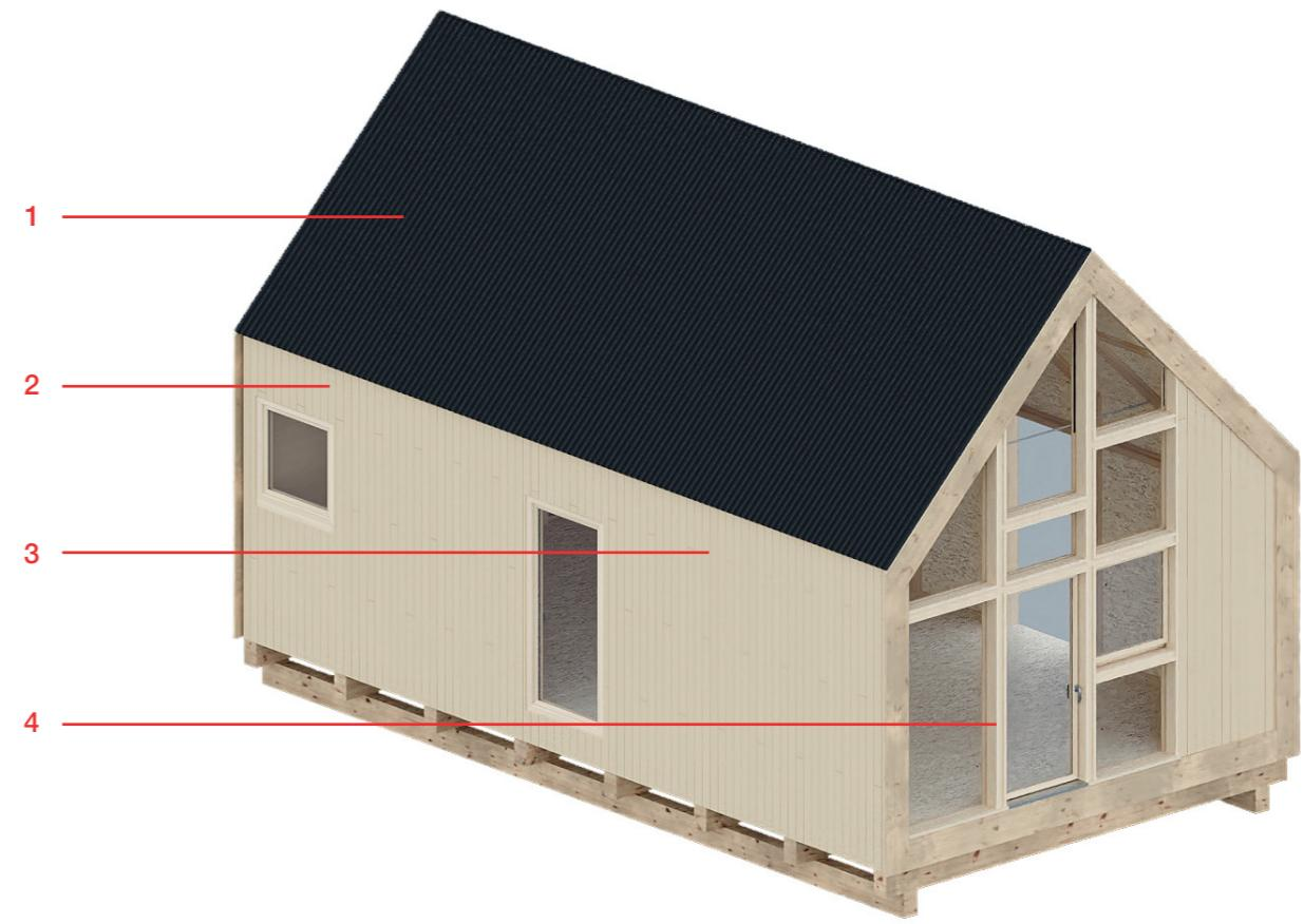
1. External roof cover made by metal sheet (crimped or corrugated). Other roofing solutions are available
